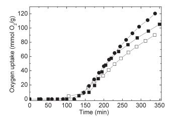
The dependencies of oxygen uptake on degradation time for unirradiated samples consisting of i-PP and CaCO<sub>3</sub> nanoparticles coated with stearic acid. (
