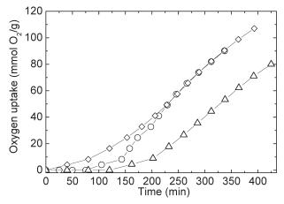
**Figure 2.**Time dependencies of oxygen uptake for irradiated at 25 kGy i-PP samples/25% CaCO<sub>3</sub> coated nanoparticles. (○) control; (△) 10% loading; (◇) 25% loading.
